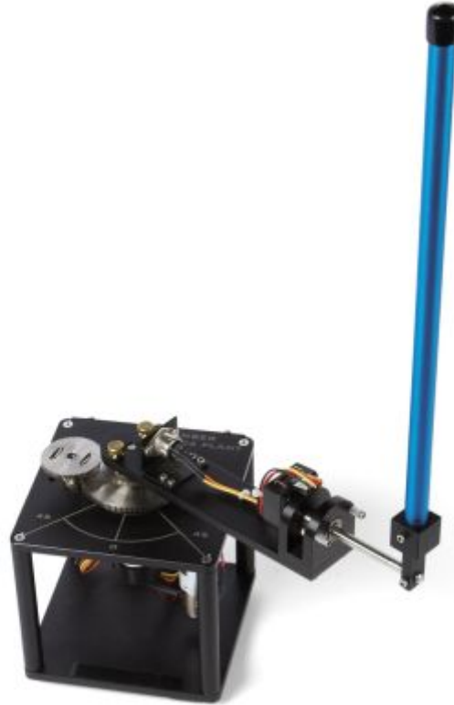
Figure 3: SRV02 ROTPEN system
