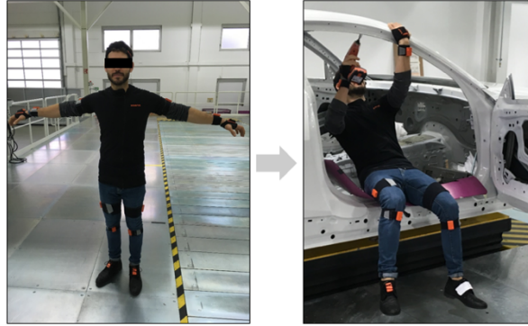
Figure 6: Xsens suit calibration and test in real environment
